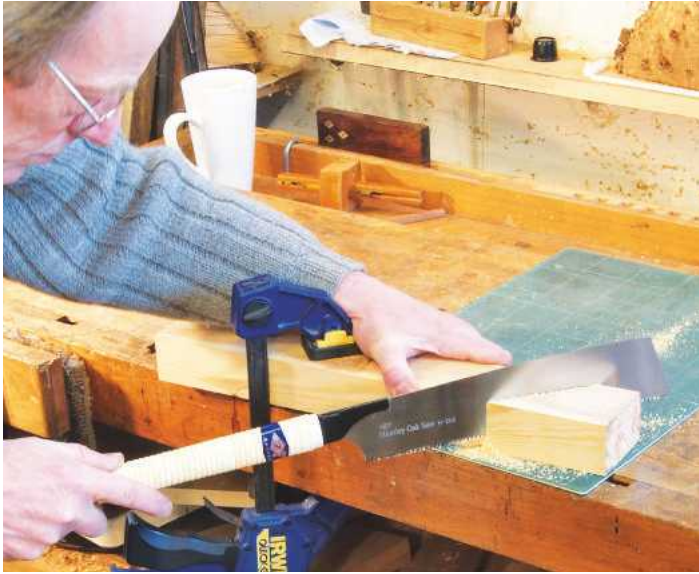
▲ Pic.2 Clamp and saw to the line, making sure your kerf is always in the waste
